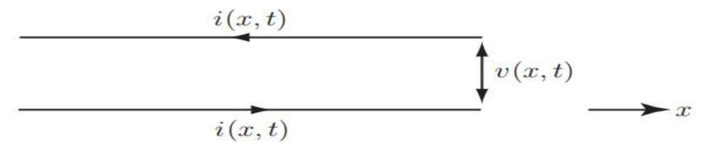
It is possible to show, using basic laws of electrical circuit theory, that the electrical current
