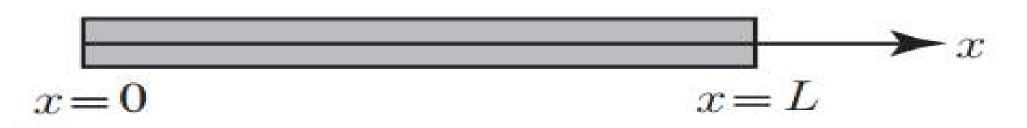
Imagine that the bar is thermally insulated laterally and is sufficiently thin that heat flows (by conduction) only in the x-direction. Then the temperature u at any point in the bar depend only on the x-coordinate of the point and the time t.By applying the principle of conservation of energy it can be shown that u(x, t) satisfies the PDE
