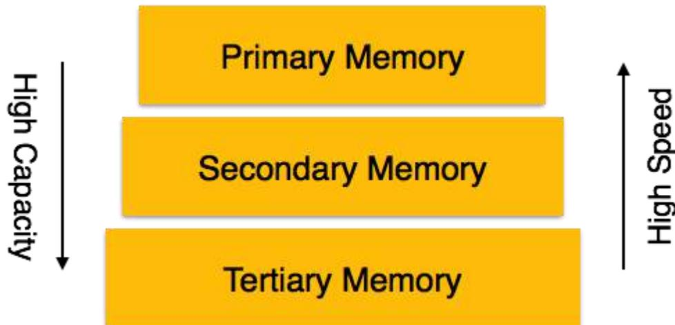
**Primary Storage** – The memory storage that is directly accessible to the CPU comes under this category. CPU's internal memory (registers), fast memory (cache), and main memory (RAM) are directly accessible to the CPU, as they are all placed on the motherboard or CPU chipset. This storage is typically very small, ultra-fast, and volatile. Primary storage requires continuous power supply in order to maintain its state. In case of a power failure, all its data is lost.
